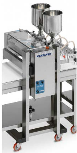
Volumetric pneumatic dosing unit with valves to control the suction and dosing of the product. Possibility of using very thick products with big pieces of particles.
